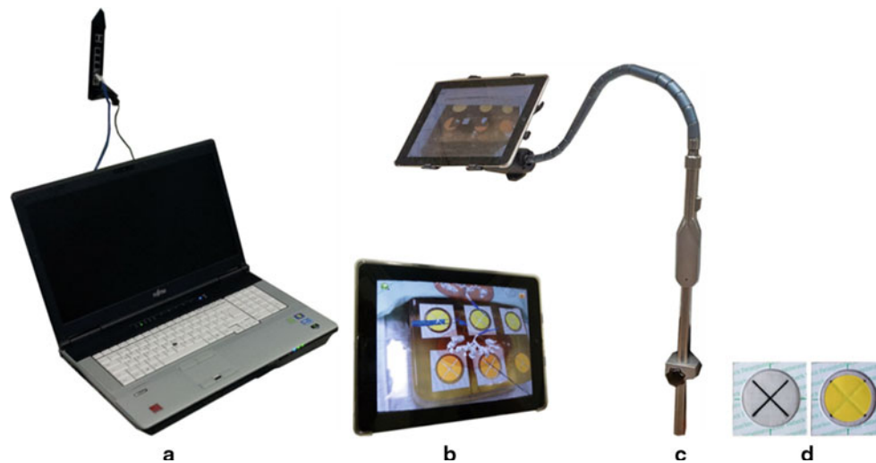
Fig. 2 The components of the navigation system: a the navigation server, b Apple iPad as mobile display, c tablet fixation on a flexible endoscope stand, d radio-dense navigation markers, optionally attached with color labels for a more robust localization
