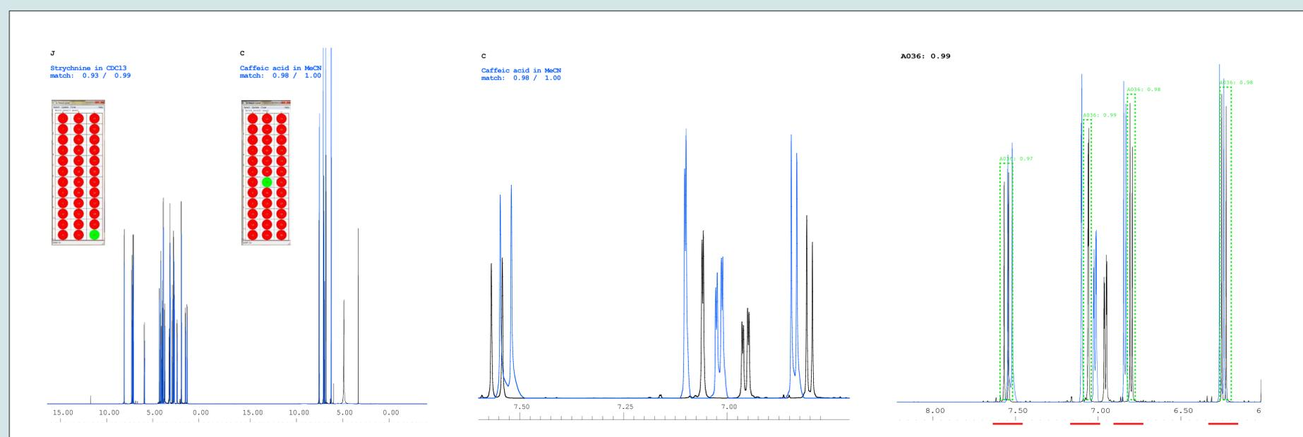
When matching an unknown against a database a visual presentation of the match percentages appears as a table of colored dots - in this case two compounds are matched. Pressing the green dot superimpose the unknown and the hit for manual inspection
