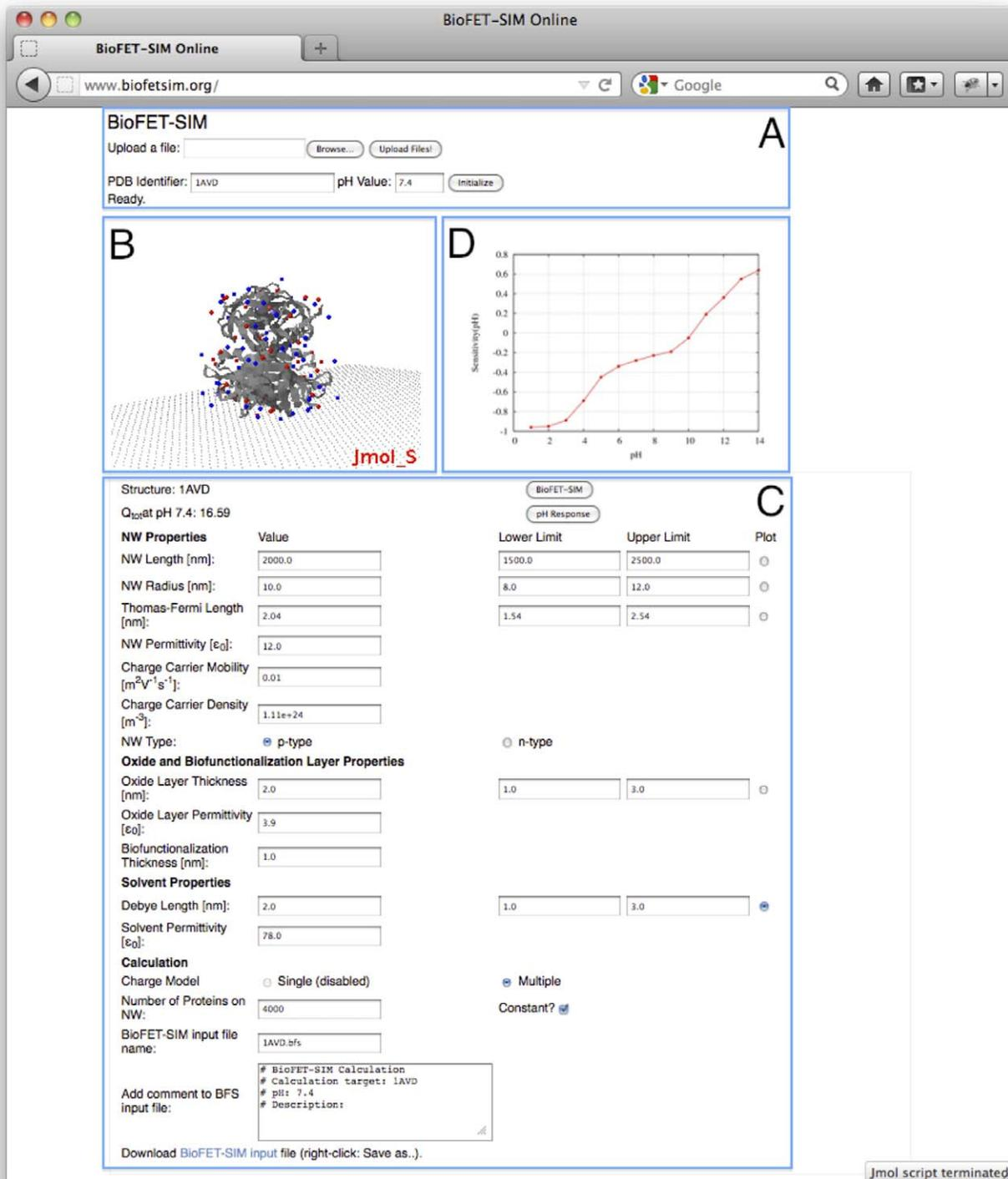
**Figure 1. BioFET-SIM Web Interface.** A: Upload or request of protein structure and pH setting. B: Jmol visualization of protein on nanowire surface. C: BioFET-SIM parameter section. D: BioFET-SIM calculation result. doi:10.1371/journal.pone.0045379.g001
