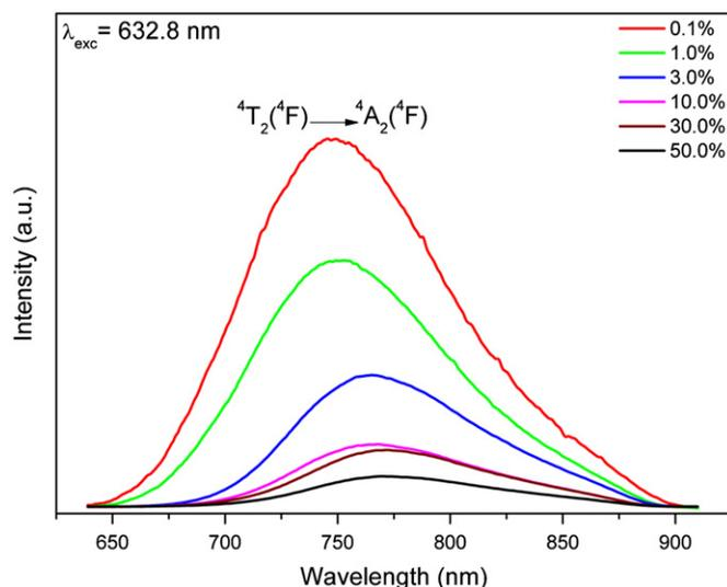
**Fig. 2.** Photoluminescence spectra at 300 K of  $\text{Cs}_2\text{NaAlF}_6$ , with 0.1, 1.0, 3.0, 10.0, 30.0 and 50.0 at% of  $\text{Cr}^{3+}$ . (For interpretation of the references to color in this figure legend, the reader is referred to the web version of this article.)
