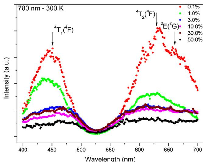
**Fig. 6.** Excitation spectra at 780 nm (300 K) of the  $\text{Cs}_2\text{NaAlF}_6$  with several concentrations of the  $\text{Cr}^{3+}$  ion. The identified transitions are labeled in the spectra.
