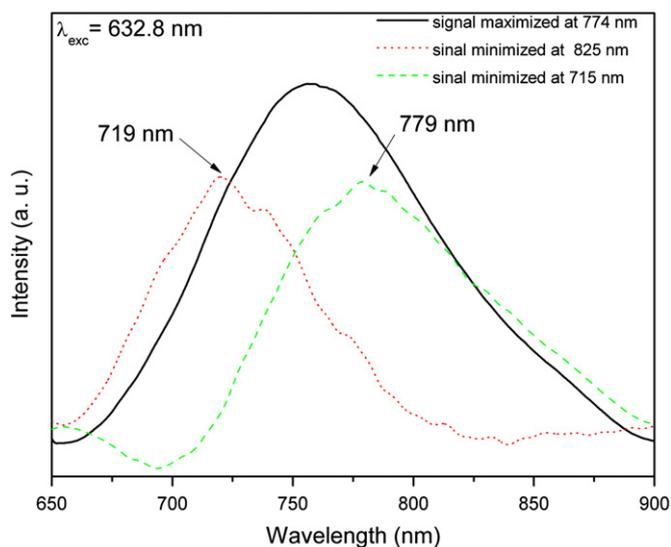
Fig. 4.  $\text{Cs}_2\text{NaAlF}_6$  luminescence spectra at 300 K with 0.1 at% of  $\text{Cr}^{3+}$ . (For interpretation of the references to color in this figure legend, the reader is referred to the web version of this article.)
