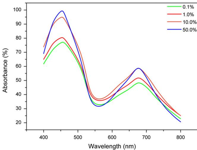
Fig. 7. Absorption spectra at 300 K of the  $\text{Cs}_2\text{NaAlF}_6$  with the concentrations of 0.1, 1.0, 10.0 and 50.0 at% of  $\text{Cr}^{3+}$ .
