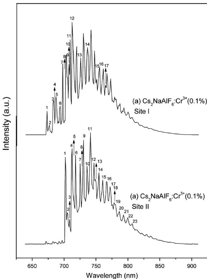
Fig. 8. Emission spectra of the  $\text{Cs}_2\text{NaAlF}_6$  with 0.1 at% of  $\text{Cr}^{3+}$  as impurity at 5 K. (a) Spectrum obtained with 672 nm zero-phonon line maximized and in (b) with the line minimized at 672 nm.
