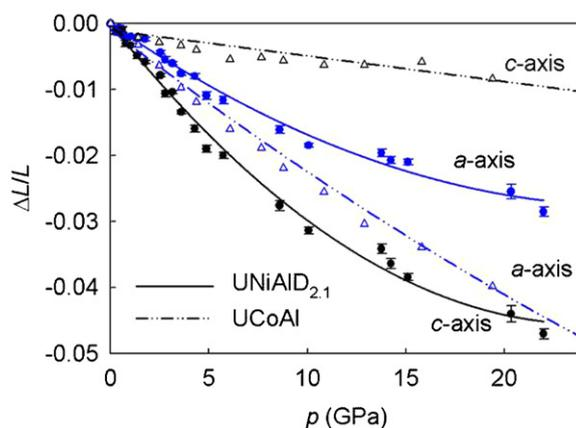
Fig. 1. Pressure variations of the relative change of the lattice parameters *a* and *c* for UNiAlD<sub>2.1</sub> compared with UCoAl [4].
