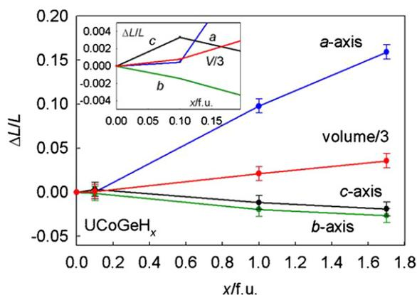
**Fig. 4.** Relative changes of lattice parameters  $a$ ,  $b$ ,  $c$  and volume  $V$  for UCoGe as a function of H concentration. The lattice parameters of hexagonal hydrides of UCoGe were recalculated for the orthorhombic representation.
