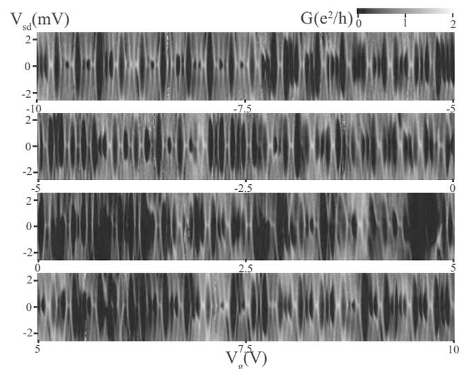
FIG. 1. Bias spectroscopy plot of a SWCNT QD for  $-10 \text{ V} < V_g < 10 \text{ V}$ . The Coulomb diamonds are seen for almost every added electron (285), and 88 odd-occupancy Coulomb blockade diamonds exhibit a zero-bias Kondo resonance.
