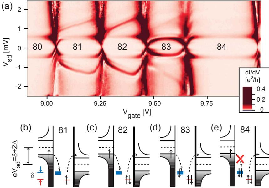
FIG. 3. (Color online) Device B. (a) Detailed bias spectroscopy at  $T=0.3$  K of one four-electron shell [dashed blue rectangle in Fig. 2(b)]. [(b)–(e)] Schematic energy diagrams illustrating inelastic cotunneling processes relevant for fillings of 1–4 electrons in a shell, e.g., corresponding to charge states 81–84. The thick blue (thin red) level represents the strongly (weakly) coupled orbital, which both are coupled more weakly to the right electrode (drain) shown by a thicker barrier.
