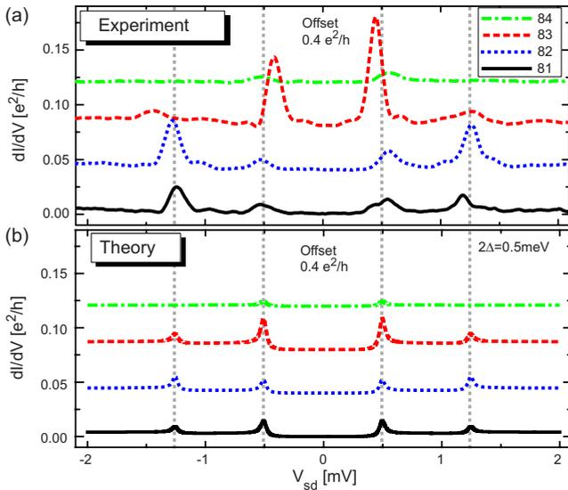
FIG. 4. (Color online) Comparison of (a) measured and (b) calculated conductance versus  $V_{sd}$  in the center of diamonds 81–84 in Fig. 3(a). In the calculation  $\delta = 3\Delta$ ,  $k_B T = 0.03$  meV and addition energies (12.6, 12.6, 10.8, and 20.7) meV extracted from the width of the diamonds 81–84 have been used.
