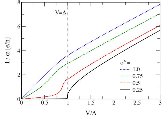
FIG. 5. (Color online) Current  $I/\alpha$  for a symmetrically coupled quantum dot occupied by an odd number of electron where the spin is treated classically. The coupling strengths are chosen  $\sigma^s \equiv \pi\nu_F W^s/2 = 1, 0.75, 0.5, 0.25$  similarly to Fig. 3.
