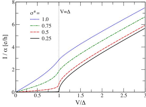
FIG. 3. (Color online) Current  $I/\alpha$  for the spinless dot (even occupation) with equal dimensionless cotunneling amplitudes to S and N given by, respectively,  $\sigma^e \equiv \pi\nu_F W^e/2 = 1, 0.75, 0.5, 0.25$ , corresponding to a cotunnel junction transmission of  $\alpha = 0.8, 0.56, 0.2, 0.015$ . Dotted line indicates the superconducting gap  $V = \Delta$ .
