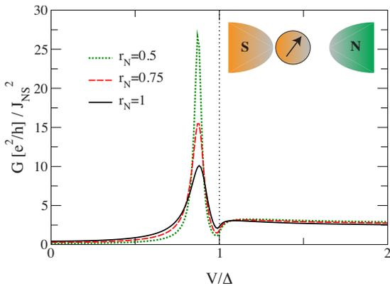
FIG. 10. (Color online) Differential conductance  $G=dI/dV$  for increasing coupling to normal lead,  $r_S=1$  and  $g_0=0.3$ . The conductance is renormalized by the “transport” coupling strength,  $J_{NS}^2$ , across the dot in order to compare the different curves. Inset: illustration of a spin state coupled to the superconducting lead, thus forming a bound state, which is probed by the normal lead.
