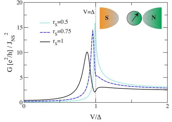
FIG. 11. (Color online) Renormalized nonlinear conductance  $G/J_{NS}^2$  for increasing coupling to the superconducting lead and  $r_N=1$ ; Inset: illustration of a spin state strongly coupled to the normal lead and thus only the superconducting DOS is probed in transport.
