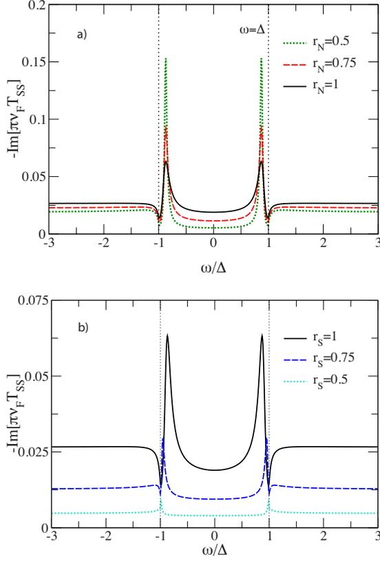
FIG. 7. (Color online) Imaginary part of the  $T$  matrix,  $-\text{Im}[\pi\nu_F T_{SS}]$ , for a spinful quantum dot asymmetrically coupled to a superconducting and normal lead with  $g_0 \equiv \pi\nu_F J_0/4 = 0.3$  leading to  $\omega_S \approx 0.8735\Delta$  for  $r_N=0$ ; (a)  $r_S=1$  is kept constant and the coupling to the normal lead  $r_N$  is changed; (b)  $r_N=1$  is kept constant and the coupling to the superconducting lead is reduced.
