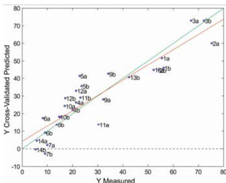
**Figure 1.** Measured vs. predicted plot of the final PLS model using 7 latent variables. The green line indicates a perfect regression. The red line indicates the regression of the PLS model. R<sup>2</sup> = 0.828, RMSEC = 2.5597 and RMSECV = 8.7027.
