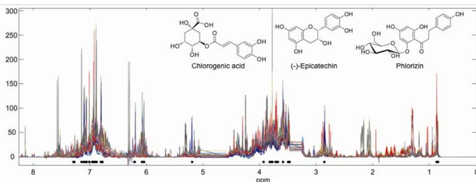
**Figure 2.** Overlaid <sup>1</sup>H NMR spectra of all 28 samples. The chemical shift intervals used in the final PLS model are indicated with black dots. Compounds identified from these chemical shift intervals are shown.
