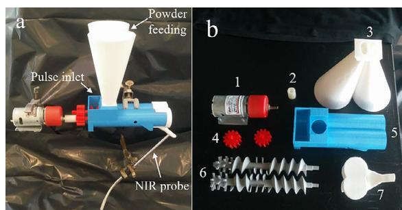
**Fig. 1.** a) The assembled experimental setup b) The experimental setup disassembled (1: Motor for rotating the twin screws, 2: Connection part between motor and sprocket, 3: Hopper with two feeding funnels, 4: Sprockets connecting active and passive screw, 5: Twin screw chamber, 6: Screw design, 7: Powder outlet).
