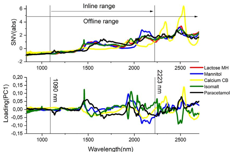
**Fig. 3.** The spectral difference of materials. Above: the SNV treated spectra of each material. Below: The spectral difference between each tracer and the carrier (lactose monohydrate) illustrated by loadings.
