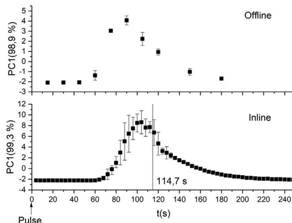
**Fig. 2.** An illustration of RTD profile for pulse experiment using mannitol as tracer. The offline data consists of 1 sample tested in triplicate at the different timestamps for the first experimental run. The inline data is an average of three consecutive experimental runs. The error bars indicate 95 % confidence interval.
