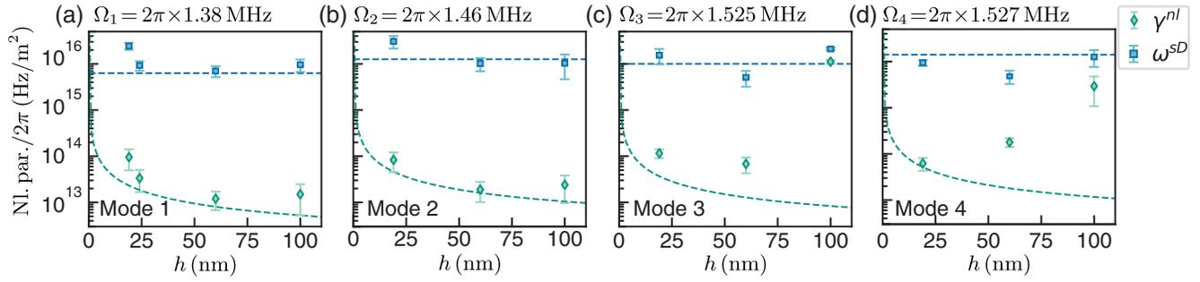
FIG. 2. Nonlinear parameters. (a)–(d) Measured nonlinear parameters as a function of membrane thickness  $h$ . Blue (green) points are the Duffing (nonlinear damping) parameters  $\omega_i^{\text{SD}}$  ( $\gamma_i^{\text{nl}}$ ), estimated from the median of each statistical ensemble. Dashed lines represent simulated values for the Duffing (blue) and nonlinear damping (green) parameters.
