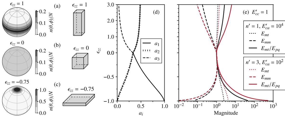
**Fig. 4.** Vertical pure shear experiment. (a)–(c) Parcel geometries and orientation distributions  $n(\theta, \phi)$  at vertical parcel strains of  $\epsilon_{zz} = 1$ ,  $\epsilon_{zz} = 0$  and  $\epsilon_{zz} = -0.75$ . (d) Modelled fabric eigenvalues ( $a_1, a_2, a_3$ ) using the spectral grain rotation model. (e) Bulk directional enhancement factors given the modelled orientation distribution  $n(\theta, \phi)$  for special cases of  $E'_{cc}$  and  $E'_{ca}$  (see main text).
