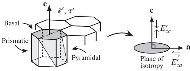
**Fig. 1.** Left: Monocrystal lattice composed of hexagonal cells. Three crystallographic planes are highlighted in gray, where the  $c$ -axis indicates the basal-plane normal direction. Right: Monocrystal modelled as a transversely isotropic material with symmetry axis  $\mathbf{c}$  and longitudinal ( $E'_{cc}$ ) and shear ( $E'_{ca}$ ) enhancement factors w.r.t.  $\mathbf{c}$ . The transverse direction,  $\mathbf{a}$ , lies in the plane of isotropy ( $\mathbf{a} \perp \mathbf{c}$ ).
