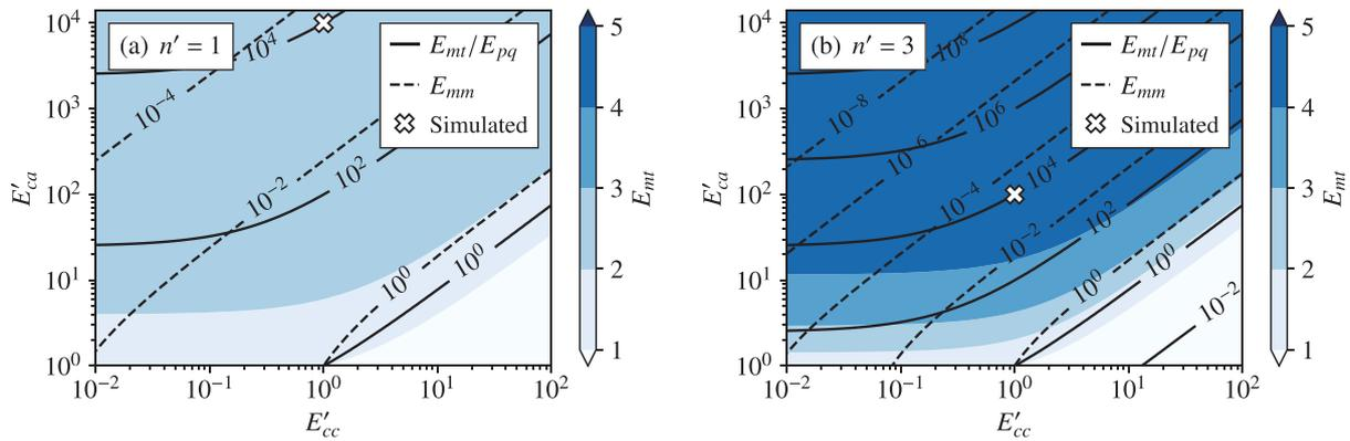
**Fig. 3.** Bulk enhancement factors  $E_{mt}$  (blue-filled contours),  $E_{mmm}$  (dashed contours) and  $E_{mt}/E_{pq}$  (solid contours) for a unidirectional orientation fabric,  $\mathbf{c} = \mathbf{m}$ , as a function of the grain enhancement factors  $E'_{cc}$  and  $E'_{ca}$  in the case of the (a) linear and (b) non-linear grain rheology. Crosses indicate the grain parameters used to model the bulk enhancement factors of an evolving fabric (Fig. 4).
