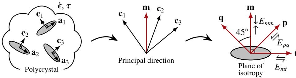
Fig. 2. Axisymmetric polycrystal with longitudinal ( $E_{mm}$ ), shear ( $E_{mt}$ ) and  $45^\circ$ -shear ( $E_{pq}$ ) bulk enhancement factors w.r.t. the symmetry axis  $\mathbf{m}$ . The transverse direction,  $\mathbf{t}$ , lies in the plane of isotropy ( $\mathbf{t} \perp \mathbf{m}$ ), while  $\mathbf{p}$  is oriented at  $45^\circ$  to  $\mathbf{m}$  and  $\mathbf{p} \perp \mathbf{q}$ .
