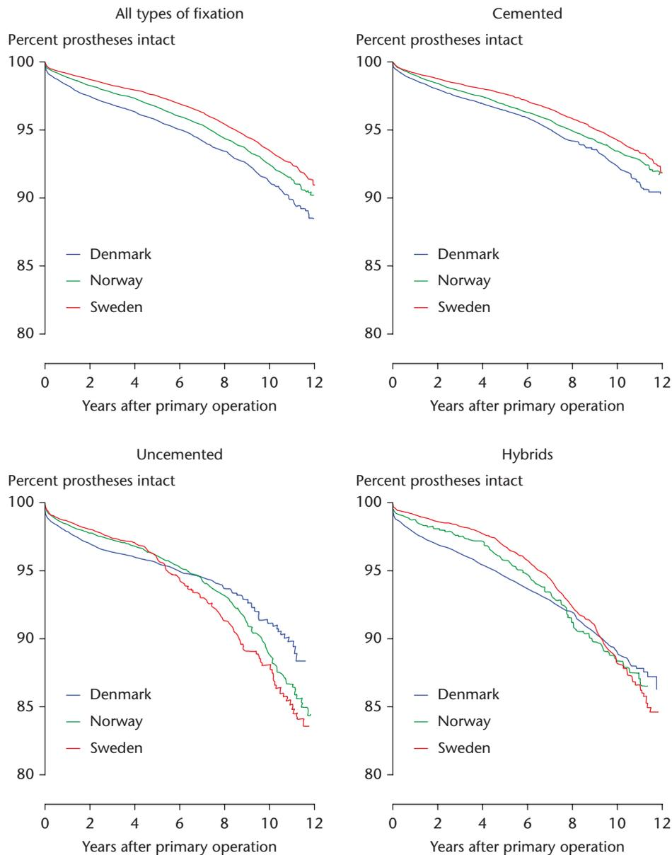
**Fig. 1** Kaplan-Meier estimated curves until revision for any cause, for primary total hip replacements (THAs) in Denmark, Sweden, and Norway 1995–2006. Curves are given for all THAs and also for those classified according to fixation technique as cemented, uncemented, and hybrids (uncemented cup/cemented stem).
