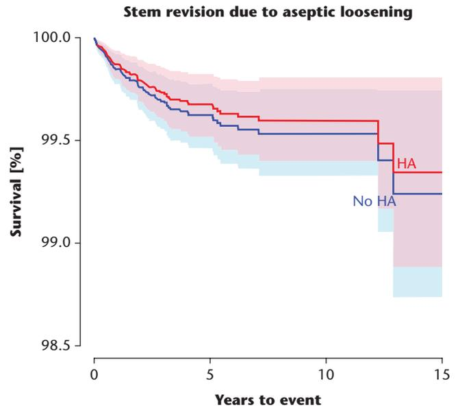
**Fig. 3** Survival of non-HA-coated and HA-coated Bimetric stems for females aged 60–74 with a diagnosis of osteoarthritis, with the endpoint stem revision for aseptic loosening in an adjusted Cox regression model.
