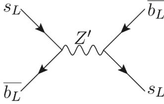
**Figure 1.** Feynman diagram of the tree-level  $Z'$  contribution to  $B_s - \overline{B}_s$  mixing.
