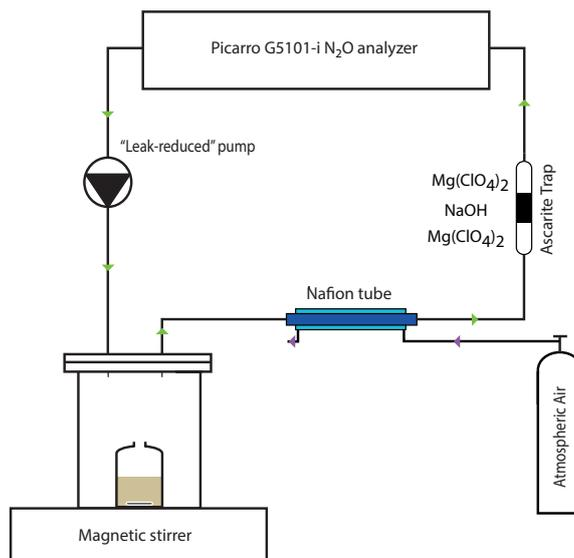
**Figure 1.** Simplified schematic of the incubation setup. The green and the purple arrows show the flow direction of the measuring gas and the purge gas, respectively.
