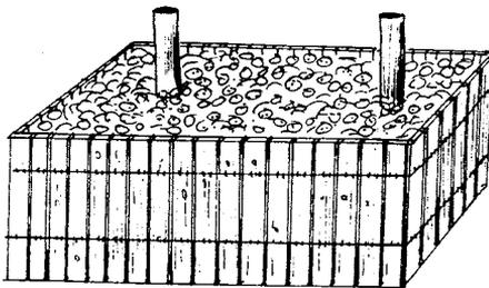
5. Large containers may be provided with loosely inserted 'chimneys' to improve ventilation of the inner part of the container.
