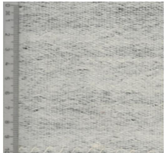
Figure 6.1.7. (left) 2/1 twill, with an average of 6 warp threads and 4 weft threads per cm. The top half shows the twill structure, while the lower half shows the reverse side with the tabby structure (photo: CTR).
