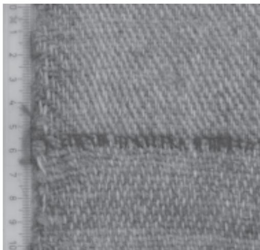
Figure 6.1.8. (right) 2/2 twill, with an average of 14.6 warp threads and 14.6 weft threads per cm (photo: CTR).
