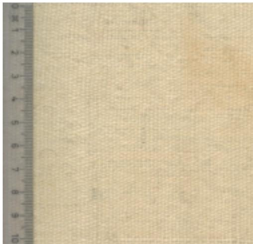
Figure 6.1.6. (right) Weft faced tabby, with an average of 5.8 warp threads and 14.8 weft threads per cm (wool fabric) (photo: CTR).
