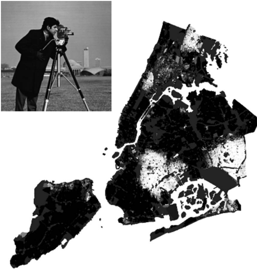
FIG. 2.—Illustration of edge detection algorithm applied to the proportion of black residents in each census block in New York City with inset of gray-scale image.
