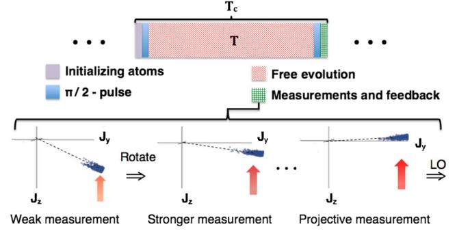
FIG. 2 (color online). Operation of an atomic clock. A clock cycle of duration  $T_c$  starts with initializing the atoms and ends with the measurements and feedback on the LO. The bottom part of the figure shows the adaptive protocol consisting of a series of weak measurements with intermediate feedback. The feedback seeks to rotate the atomic state to have mean spin almost along the  $y$  axis before the final projective measurement and subsequent feedback on the LO.
