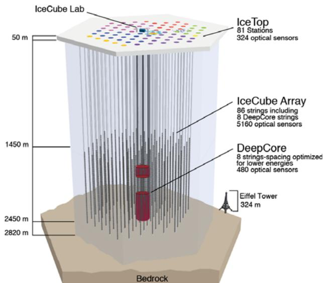
Figure 1: Layout of the IceCube detector, including the surface array (IceTop) and low energy extension (DeepCore).
