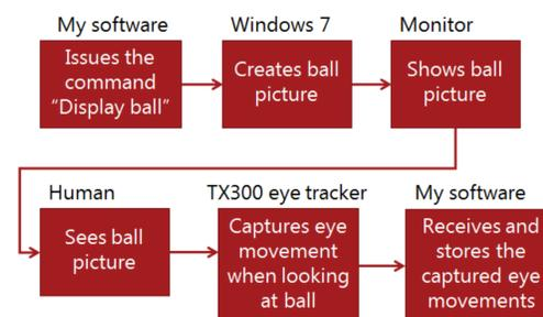
Figure 3: The flow of command when displaying data
