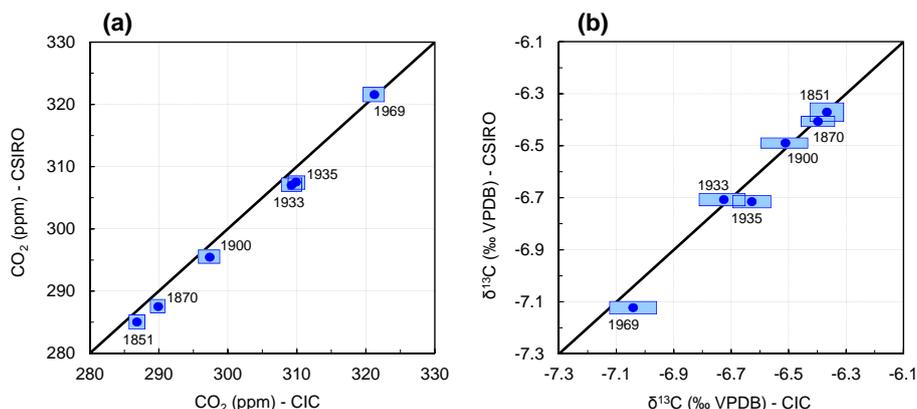
**Figure 7.** Laboratory intercomparison measurements between CIC and CSIRO of Law Dome ice core samples covering the recent past (1851–1969 AD). CO<sub>2</sub> mixing ratios (a) and δ<sup>13</sup>C-CO<sub>2</sub> values (b) measured at CIC (*x* axis) and CSIRO (*y* axis; Rubino et al., 2013) are shown. Blue boxes indicate 1σ uncertainties defined for each laboratory by the respective side length.
