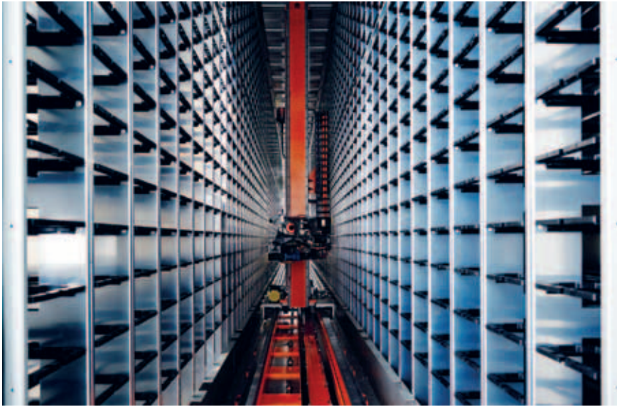
Plate 8 New freezer with robotic arm providing storage space for future samples at the Danish National Biobank. Photo: SSI
