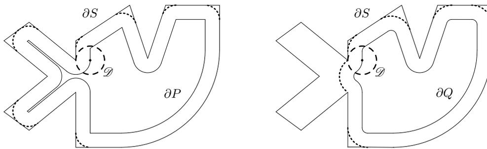
■ **Figure 3** A pocket bounded by  $\partial S$ . To the left is shown the boundary  $\partial P$  of the inwards offset of  $S$  by  $r$ . To the right is shown the boundary  $\partial Q$  of the maximum subset with bounded convex curvature of  $P$ . The dotted arcs in the corners show the boundary of the material in  $S$  that cannot be removed by  $\mathcal{D}$  using the two toolpaths.
