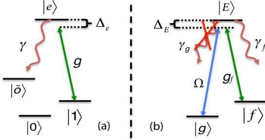
FIG. 1 (color online). (a) Level structure of the qubit atoms. Only state  $|1\rangle$  couples to the cavity and we assume that the excited level decays to some level  $|\tilde{0}\rangle$ , possibly identical to  $|f\rangle$  or  $|0\rangle$ . (b) Level structure of the auxiliary atom and the transitions driven by the weak laser ( $\Omega$ ) and the cavity ( $g_f$ ). We assume that  $|E\rangle \leftrightarrow |f\rangle$  is a closed transition, i.e.,  $\gamma_g = 0$ .
