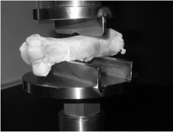
Figure 2. Three-point bending apparatus. A fourth metacarpal bone is supported on its lower side at 2 points, and compression is applied at a single point from above.
