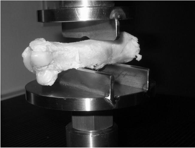
**Figure 2.** Three-point bending apparatus. A fourth metacarpal bone is supported on its lower side at 2 points, and compression is applied at a single point from above.
