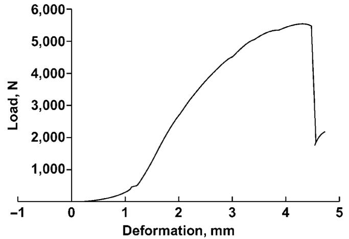
**Figure 3.** Load deformation curve for 1 individual. Load in Newtons is plotted against deformation in millimeters. The slope of the straight-line region relates to stiffness. Maximum load occurs at the breaking point (seen on the graph as the sudden drop in load) in this specimen.
