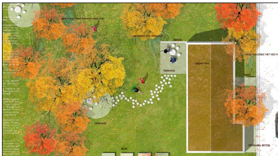
Figure 5: The storm water is primarily handled within the private lot. Part of site plan, team C. (Illustration: MASU PLANNING)
