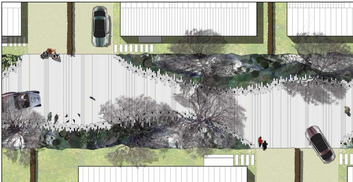
Figure 7: Team D first proposal using wadi's and private driveways to make the road and gradient sinuous. Part of site plan. (Illustration: BOGL)
