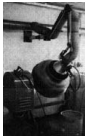
Figure A6.3. Cement mixer used for threshing, depulping, polishing, dewinging and pretreatment of fruit or seed. Fruit or seed material are tumbled together with wooden blocks, sand or gravel, and/or water depending on function. The mixer is provided with an exhaust to remove dust and wings.
