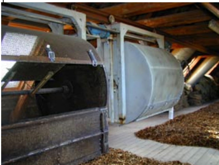
Figure A6.5. Rotating drum kiln. Danish Tree Improvement Station.
