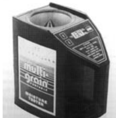
Figure A5.12. Seed moisture meter.
