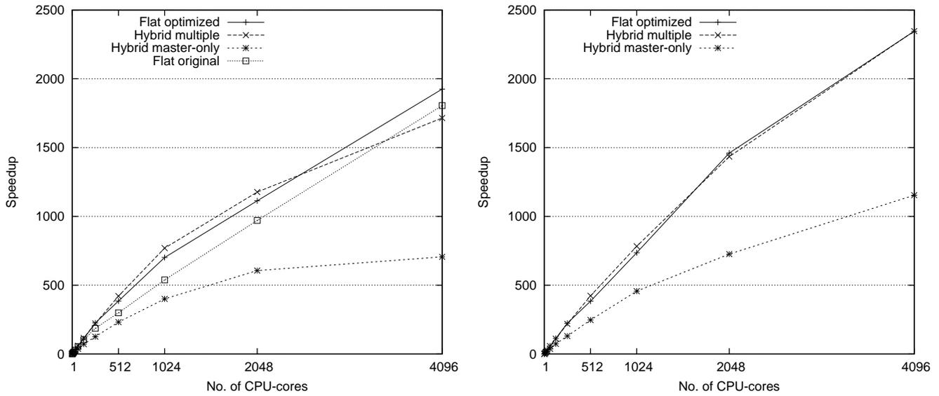
Fig. 5. Speedup of the finite-difference operation. The job consist of only 32 real-space grids all with a size of  $144^3$ . In the left graph batching is disabled and in the right graph batching is enabled using a batch-size of 8.
