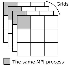
Fig. 3. Four 2D grids distributed over nine processes.
